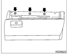
2. Open the glove box, then remove the three upper glove box screws. Remove the glove box assembly from the instrument panel to access the in-cabin microfilter cover.
